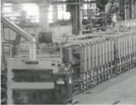
Figure 2. Continuous controlled-atmosphere furnace. (Photo courtesy of Seco/Warwick Corp.)
