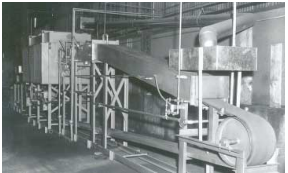
Figure 3. "Hump-back" furnace used to manufacture small assembled parts. (Photo courtesy of Seco/Warwick Corp.)
