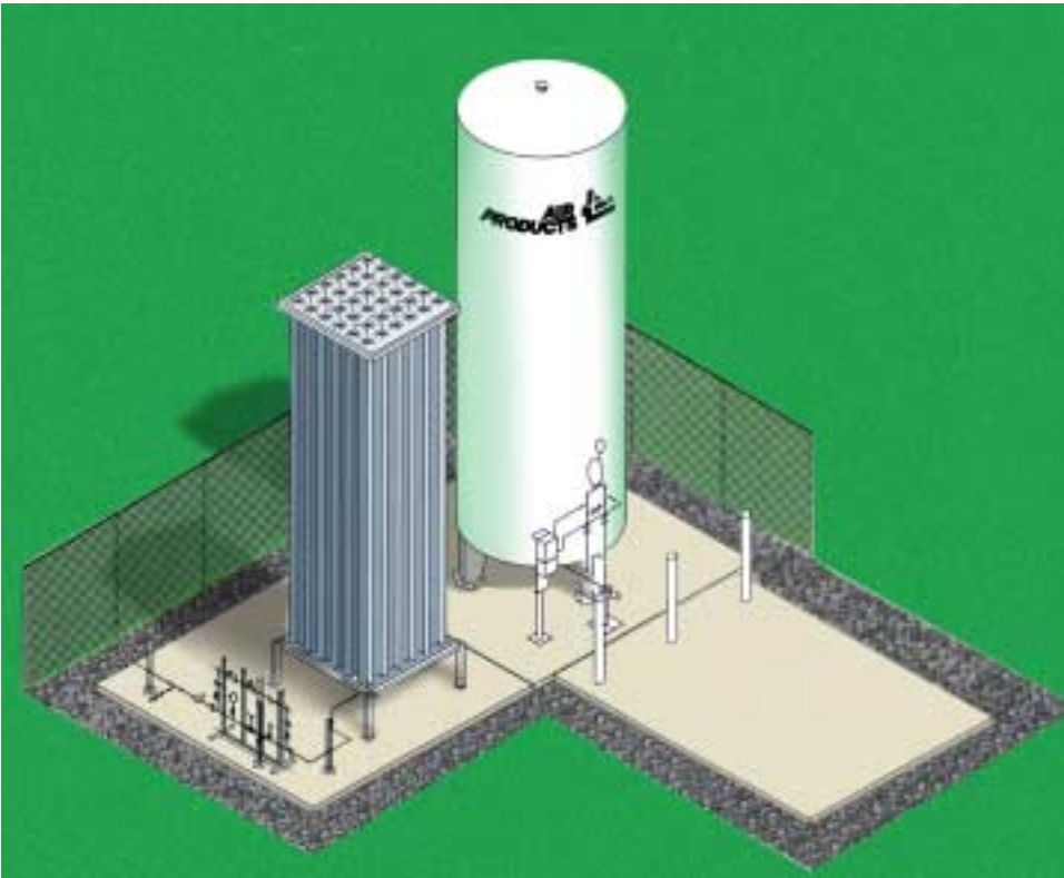
Figure 24. Schematic diagram of a typical on-site cryogenic tank system.
