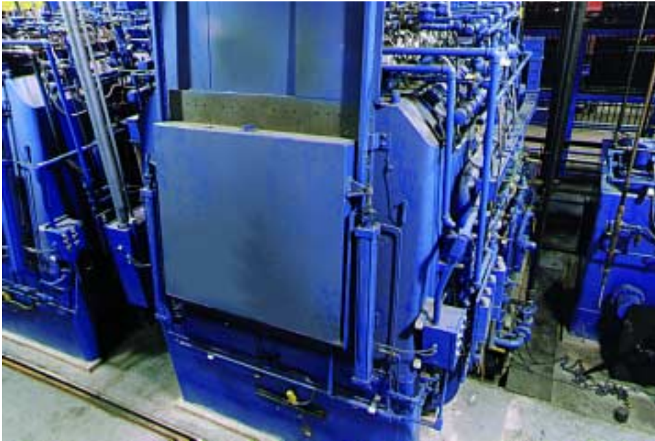
Figure 4. Batch atmosphere “box-type” furnace. (Photo courtesy of Ipsen International, Inc.)
