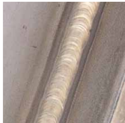
PB TIG (141) fillet in 3mm austenitic stainless steel using Inolinx® TIG gas.
