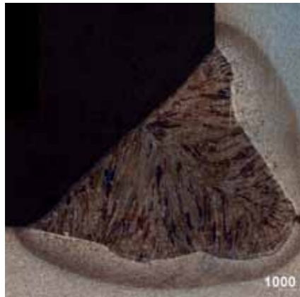
PB MAG (135) fillet in 12mm thick carbon steel using Ferrolinx® U gas.
