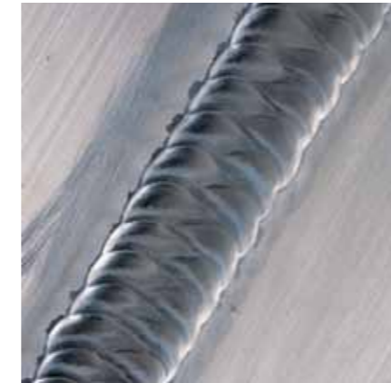
TIG butt weld in 10mm thick 4140 aluminium alloy using Alulinx® gas
